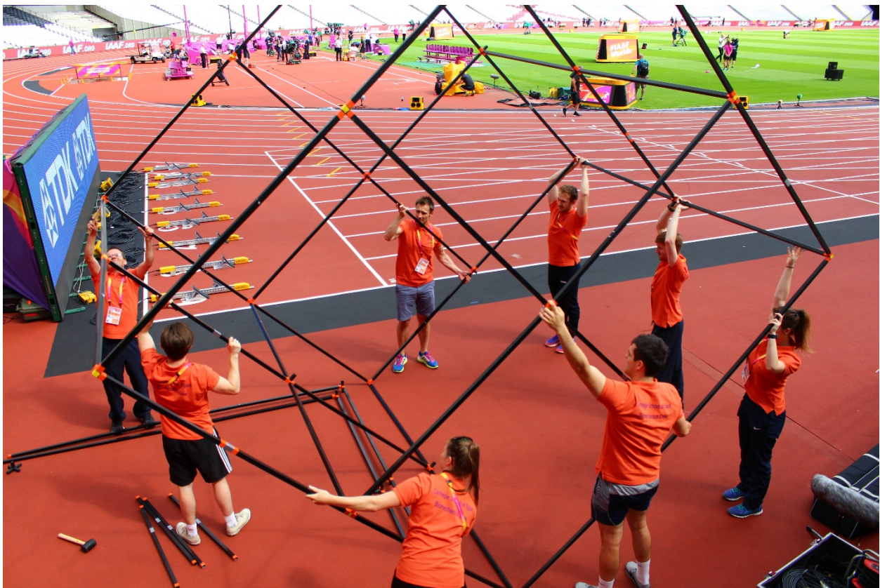
Figure 3. The calibration frame was constructed and filmed before and after the competition.
