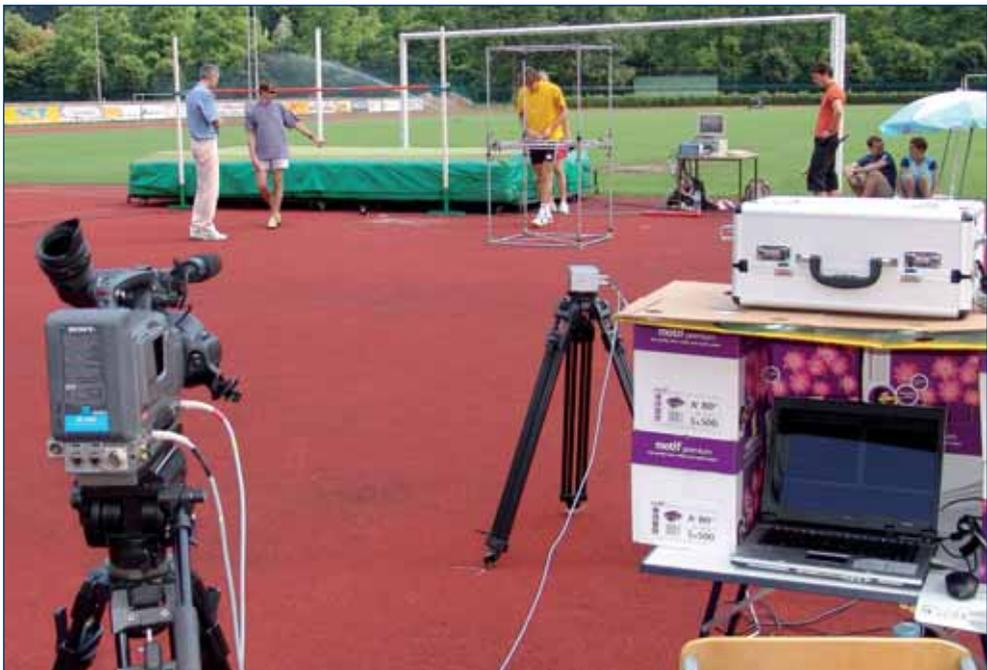
Figure 1: Measurement equipment for the 3D kinematic analysis of the high jump
