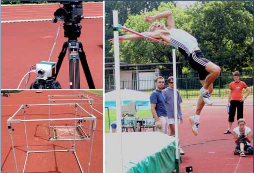
Figure 3: Measurement of the ground reaction forces on the  $y$ ,  $x$  and  $z$  axes using a force plate
